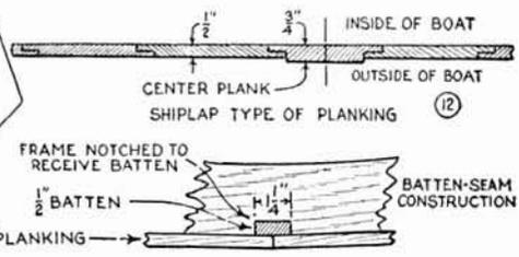
flat-head brass screws and to the sides with 1/4-in. No. 6 flat-head brass screws spaced 1 1/2 in. apart in a staggered row. Then fair off the sides, transom and stem, a job which must be done carefully to avoid leaks. At this point, select the type of bottom construction. If it is to be the batten-seam type, battens must be mortised at the proper places and the planks are fastened to the battens with 1/4-in. copper nails spaced 2 in. apart and clinched.
