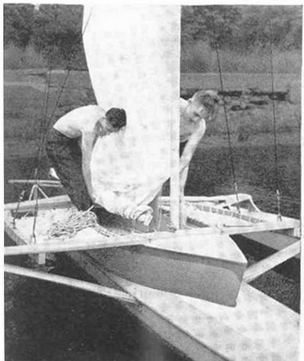
Raising the plywood centerboard, above, cuts draft of main hull to a few inches. Below, lightweight aluminum boom is easy to handle when hoisting main-sail. Note cable stays anchored to cockpit supports
