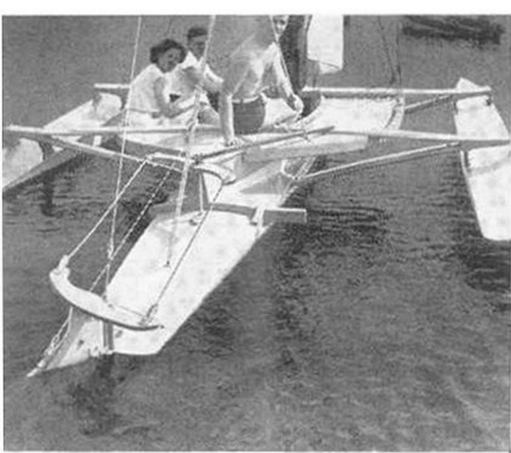
Above, stern view of Trimaran shows wooden bracket just aft of cockpit. This permits emergency mounting of outboard motor on starboard side of center hull
